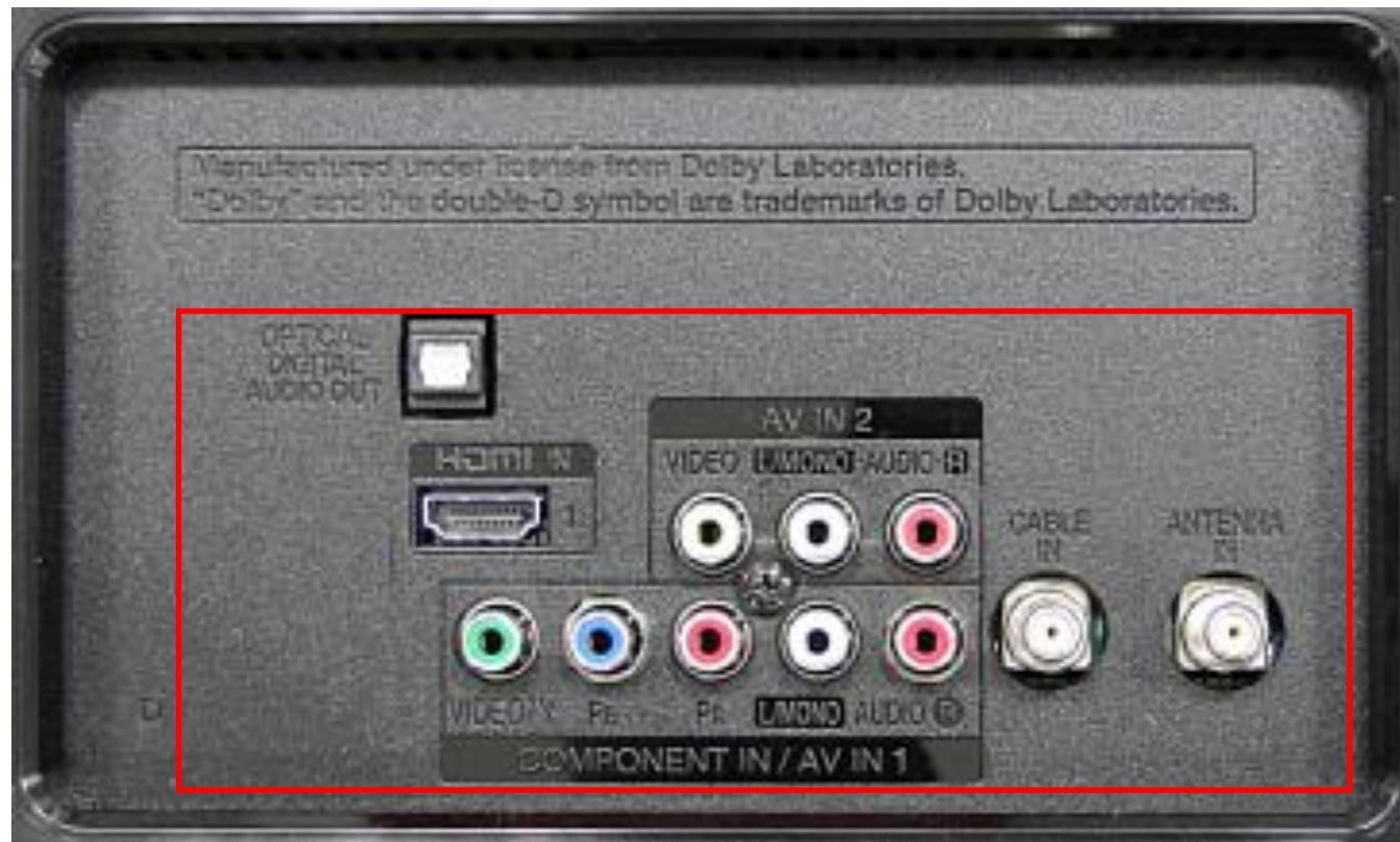
As the part connecting to the external input, check the screen condition by signal
