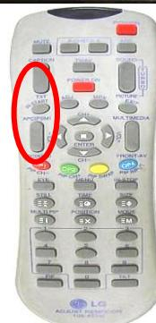
Press the IN-START with the remote controller for adjustment
