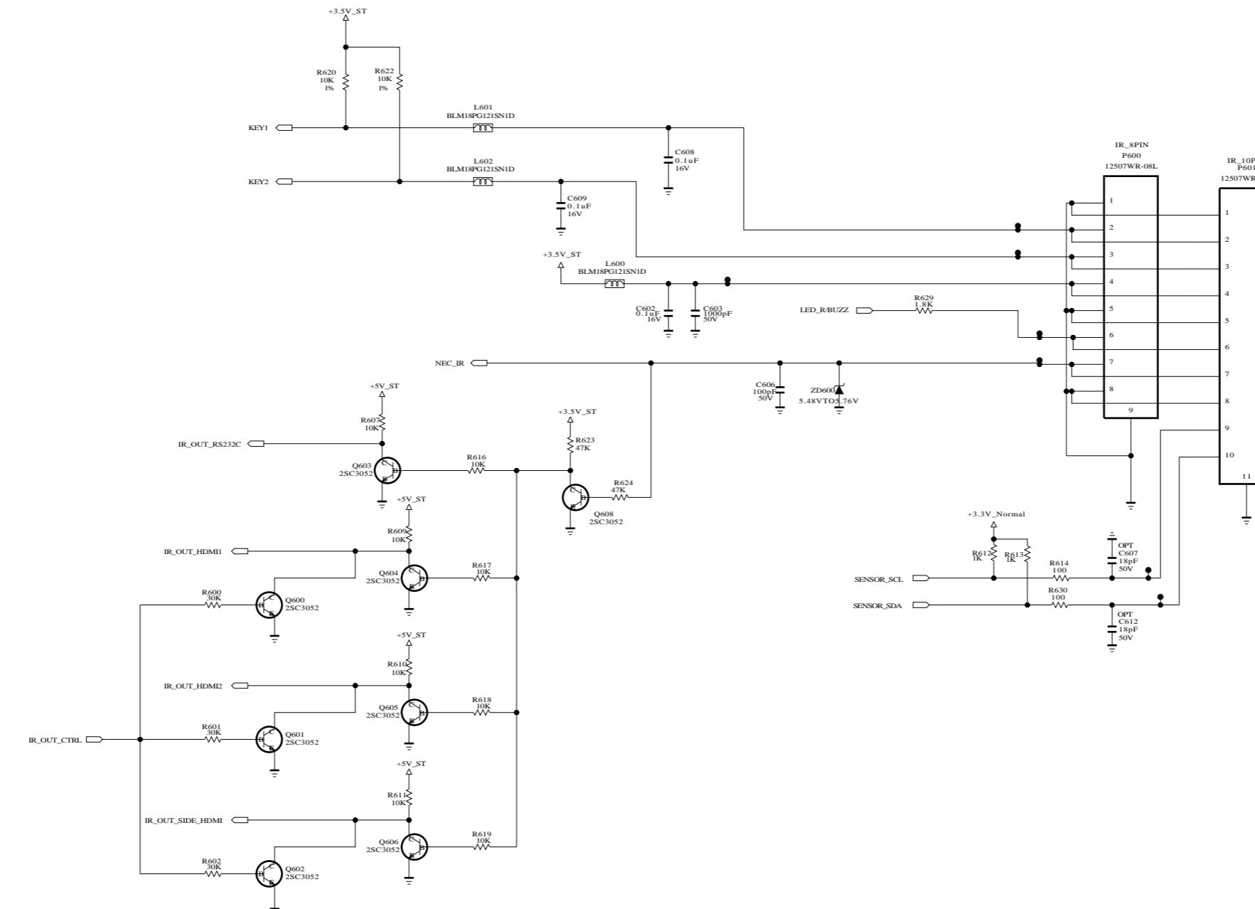
THE SYMBOL MARK OF THIS SCHEMATIC DIAGRAM INCORPORATES SPECIAL FEATURES IMPORTANT FOR PROTECTION FROM X-RADIATION. IT IS THE RESPONSIBILITY OF THE MANUFACTURER TO ENSURE THAT THE CRITICAL COMPONENTS IN THE SYMBOL MARK OF THE SCHEMATIC ARE REPLACED WITH APPROVED EQUIVALENTS.
