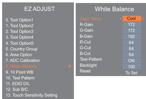
\* After you finished all adjustments, Press "In-start" key and compare Tool option and Area option value with its BOM, if it is correctly same then unplug the AC cable. If it is not same, then correct it same with BOM and unplug AC cable. For correct it to the model's module from factory Jig model.
